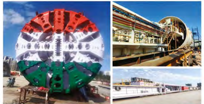
Tunnel Boring Machine for construction of Tunnel
