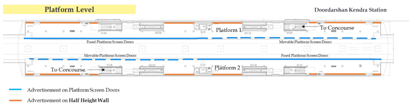
Figure 6: Typical Layout of Platform level of an Elevated Metro Station
